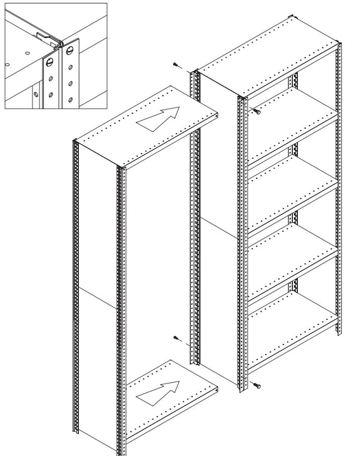
**13.** If two units are to be placed back-to-back, and you have only one back panel, the two units may share the same back panel by attaching it on the OUTSIDE of the uprights. If you have ordered two units, each with a back, you can use both backs on the INSIDE of the uprights.
