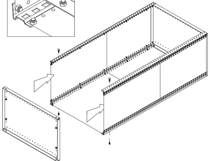
**9.** Position the shelf clips according to your desired shelf height, and place the shelves over the clips. Keep in mind, while placing the clips, that the post hole pattern of two round holes and then one square hole, repeated every 3", can greatly help in positioning the clips at the same level.
