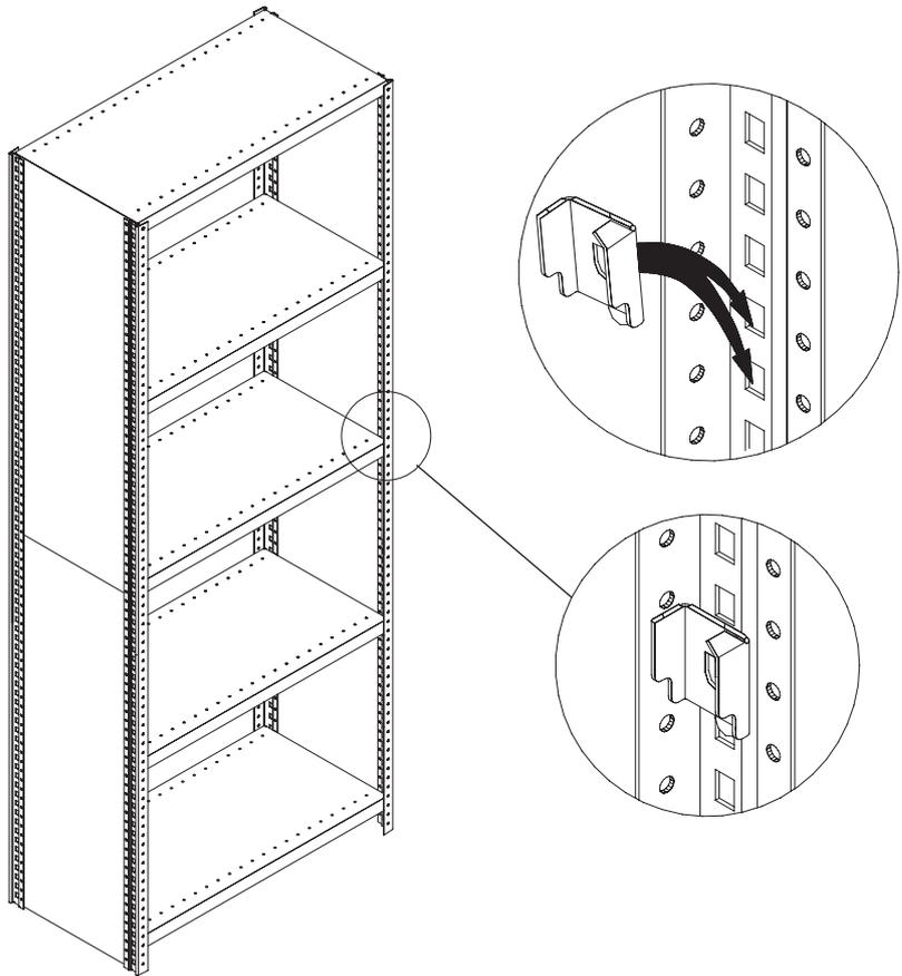
**11.** For added strength, place two  $\frac{1}{4}$ -20 x  $\frac{5}{8}$ " bolts and nuts (not included) through each corner of each shelf, and into the small holes of the upright.
