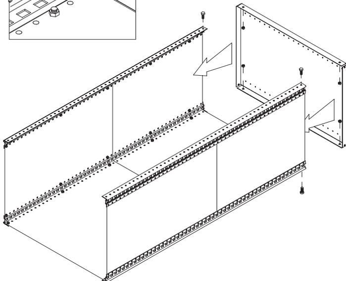
**8.** Bolt the bottom shelf using the third hole from the bottom.
